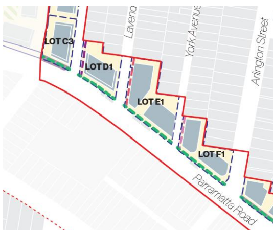
York Avenue, Lavender Street and Courland Street widening to formalise the location of the public footpaths within the public domain (Kings Bay Masterplan)
